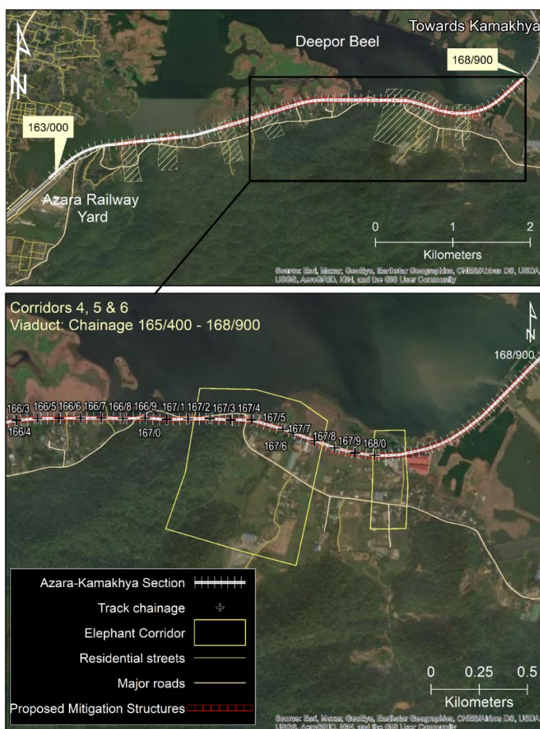
Figure 5. Railway track, elephant corridors and mitigation measures proposed by NFR and recommended by WII for doubling of railway track between chainage 165/400 – 168/900 of the Azara – Kamakhya railway line passing through the southern boundary of Deepor Beel, Guwahati, Assam.
