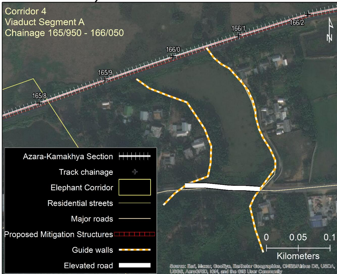
Figure 6. Additional mitigation measures recommended in the first segment (chainage 165/950 – 166/050) of the 3500 m ling viaduct on the Azara – Kamakhya railway line passing through the southern boundary of Deepor Beel, Guwahati, Assam.
