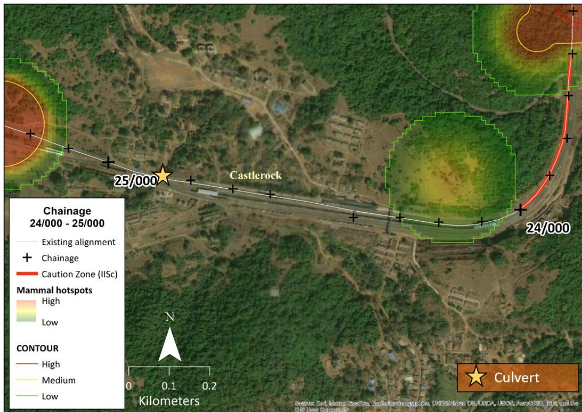
Figure 40: Locations of mitigation measures on chainage 24/000 – 25/000 to be constructed on existing and proposed railway track (NOTE: locations are approximated to the nearest chainage).
