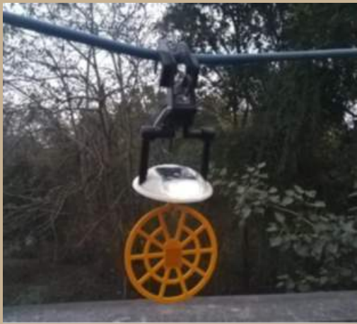
Image 12. Model Bird diverter/ reflector with rotating, reflecting and night blinking properties that has been pilot installed and field tested by Wildlife Institute of India with the assistance of power agencies in Jaisalmer.
