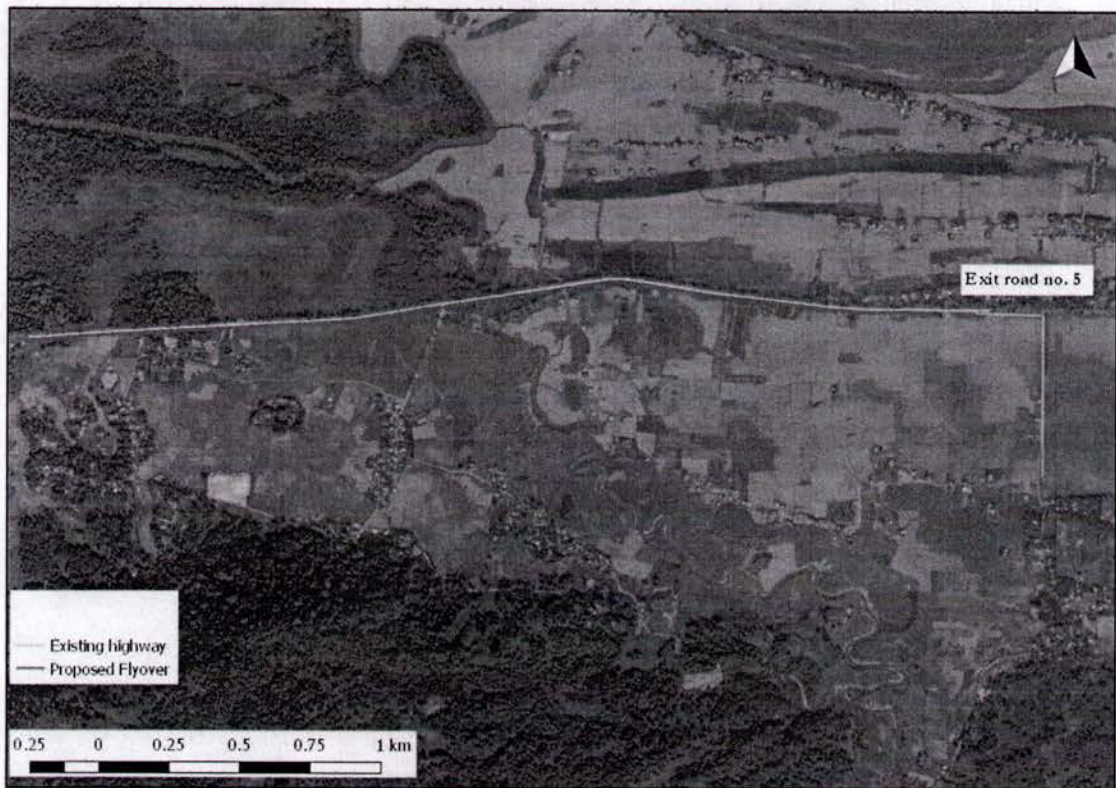
Figure 10: Exit road no. 5 linking settlements to proposed flyover (at corridor I) through existing highway.
