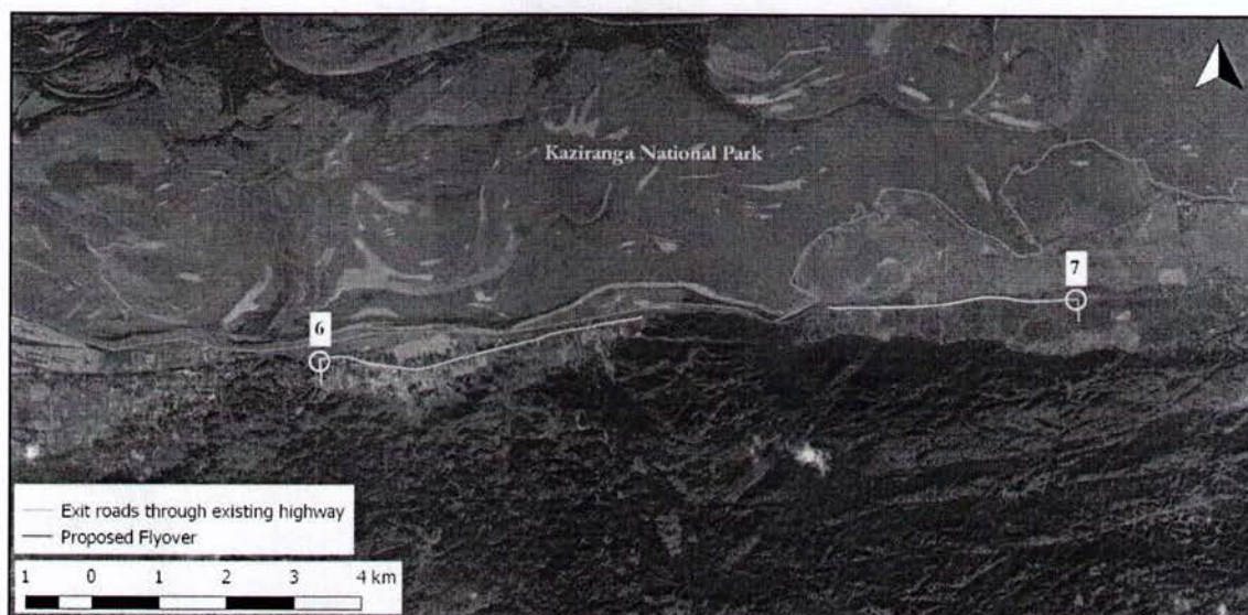
Figure 11: Proposed flyover from Na-Jan N.C. to Hathikuli with 2 road stretches connecting about 6 villages to the flyover.
